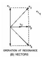
When input frequency is same as resonant frequency of the tuned circuit  $V_3$  is in phase quadrature with  $v_1$  and  $v_2$ . The resonant voltage  $v_{a1}$  and  $v_{a2}$  are equal in magnitude.
