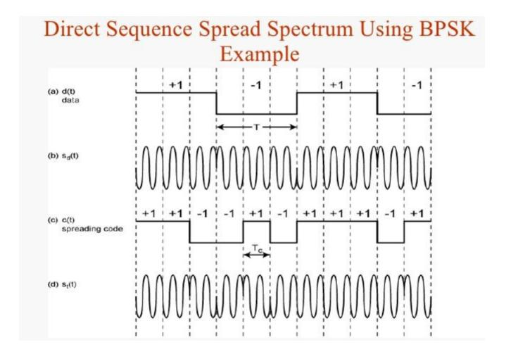
Some practical and effective uses of DSSS include the Code Division Multiple Access (CDMA) channel access method and the IEEE 802.11b specification used in Wi-Fi networks.
