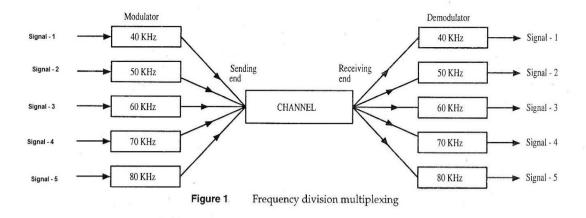
Then modulated signal are summed to produced composite multiplexed signal. The composite modulated signal is modulated by once again if necessary otherwise transmitted directly over the single channel. In receiving end individual signals are extracted from FDM signal by appropriate filtering.
