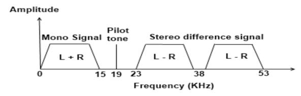
The modulating, (base-band) signal for a stero VHF F.M transmission
