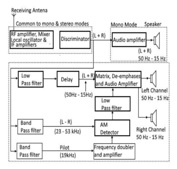
Stereo FM Receiver Block Diagram
