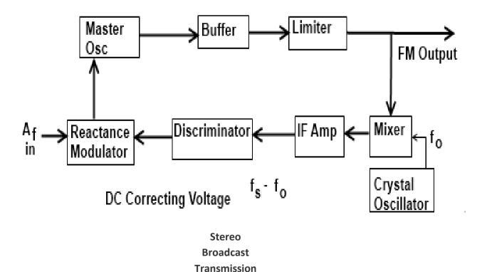
A small portion of the signal is taken from the limiter output and fed to mixer in which this signal is mixed with a signal from the crystal oscillator. The difference signal which is usually about one-tenth- to one-twentieth of the master oscillator frequency is amplified and applied to a phase
