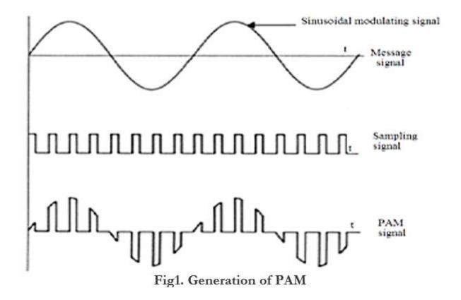
In single polarity PAM a fixed dc level is added to the signal to ensure that the pulse are always positive . In double polarity PAM the pulses appear both in positive and negative side
