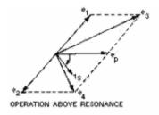
When input frequency is greater than resonant frequency phase difference between  $v_1$  and  $v_3$  is  $>90^\circ$  and phase difference between  $v_2$  and  $v_3$  is  $<90^\circ$ . From this figure the resonant  $v_{a1}$  is increased where as and  $v_{a2}$  is reduced . The RF voltage  $v_{a1}$  and  $v_{a2}$  are separately rectified by the diode  $D_1$  and  $D_2$  respectively to provide voltage  $v_{out1}$  and  $v_{out2}$ . Thus the output will be
