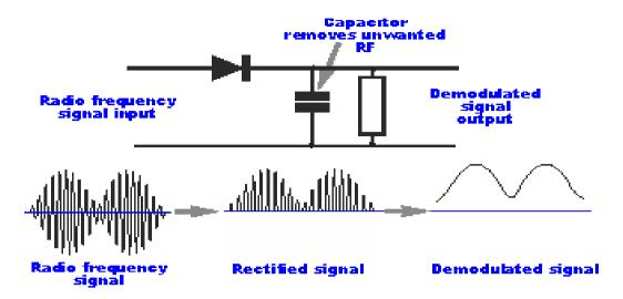
Diode detector is called envelope detector as it is recovers the audio frequency signal envelope from the composite signal. Diode detector is called linear detector as its output is proportional to the voltage of the input signal . Antenna receive different modulated wave which was transmitted by different transmitter. The desired modulated wave is selected by a tuned RF amplifier which consists of a tank circuit  $L_1 \& C_1$ .
